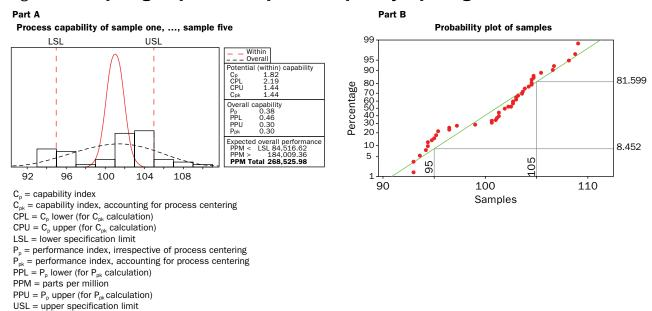
Figure 9. Reporting process capability and performance when there is no specification
